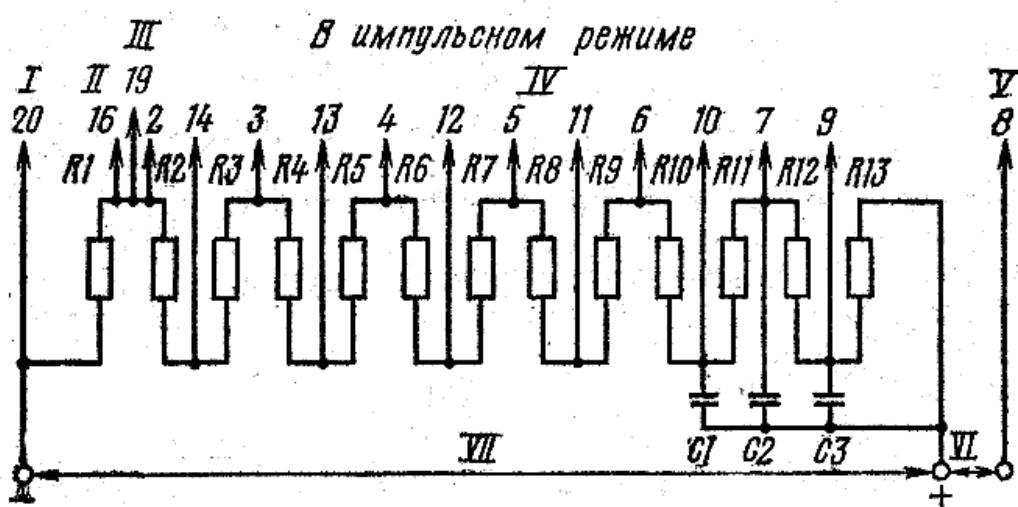
Typical voltage divider circuit photomultiplier FEU-82-82A, to operate in pulse mode. Voltage divider - uneven: R1 = 0.7R; R2 = 0.8R; R3 = 0.9R; R10 = 1.2R; R11 = 1.5R; R12 = 2.2R; R13 = (2 ... 6) R; R4 to R9 = R. Capacitors; C1 = 0.011 microF; C2 = 0.25 microF; C3 = 0.05 microF
