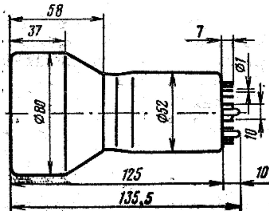
Photocathode - translucent antimony-caesium spectral response No. 4. Optical input end window diameter of 60mm cathode area. Number of amplification stages 12. Made of glass basic weight 220 g. Interconnection of electrodes and a typical voltage divider circuit to operate in static mode like FEU-81.
